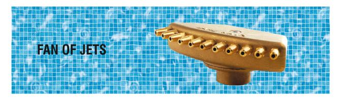
This fountain nozzle is a water manifold that houses up to 21 divergent lance jets, with 4 mm diameter jet nozzle heads. Because of the outlet angle, these jets are also parabolic, i.e. it combines both patterns: divergent fans and parabolic water jets. It is usually used in outdoor fountains and swimming pools as a secondary feature. To keep the jets compact, heights of over 5 metres are not recommended.
